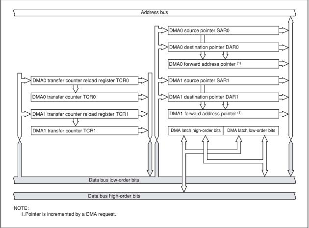
Figure 11.1 DMAC Block Diagram
